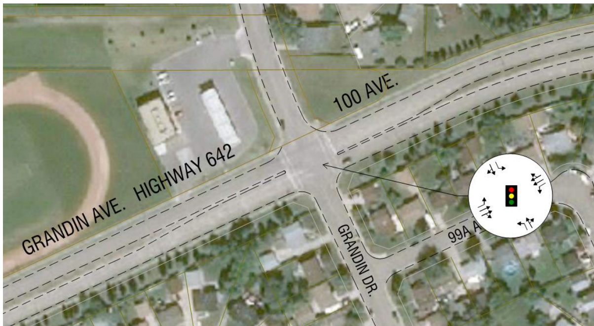
Figure 4.3: Future Intersection Configuration (Signalized – Preliminary)
